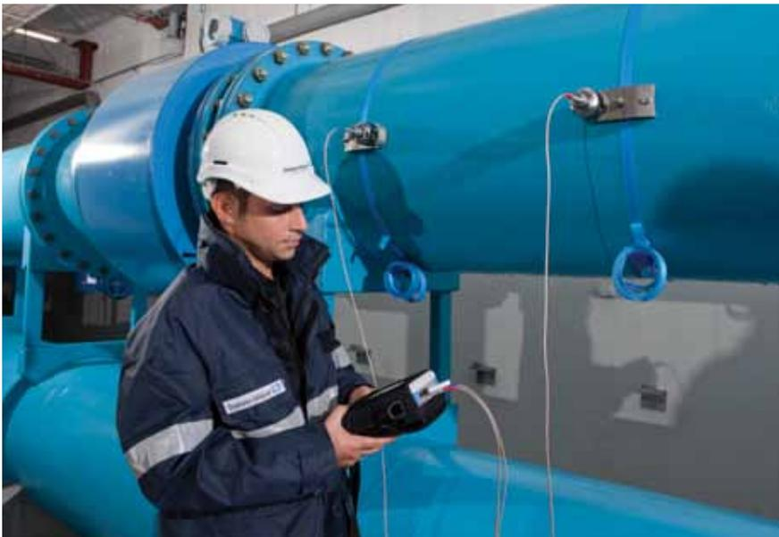
Verification of a flow measurement during live operation by an experienced service technician
